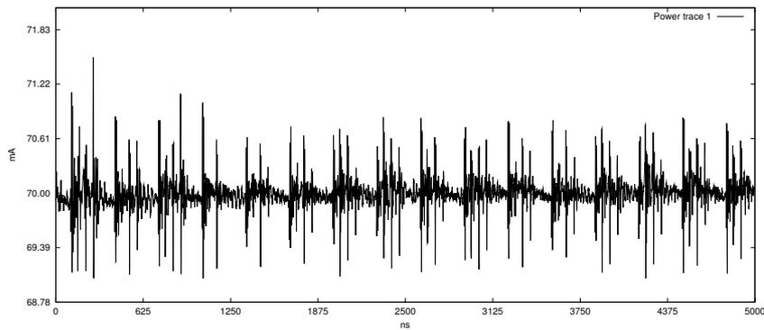
Fig. 7. Power consumption of the microcontroller encrypting  $x$ .
