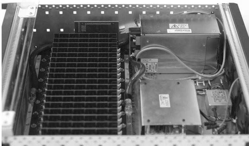
Figure 3. Complete COPACOBANA system with 20 DIMM modules
