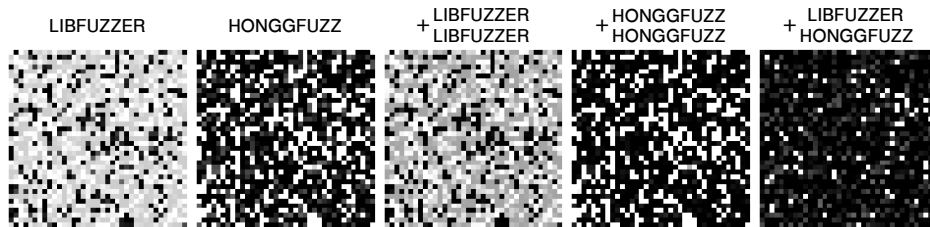
Figure 3: Actual probabilities (first two images) and predicted synchronized probabilities for the branches in FREETYPE2 when combining HONGGFUZZ and LIBFUZZER . Every cell represents a single branch. The alpha value of a cell represents the probability that this branch will be solved by this fuzzer (or fuzzer combination). For illustration purposes, we only selected an excerpt of all branches to make the differences visually distinguishable.
